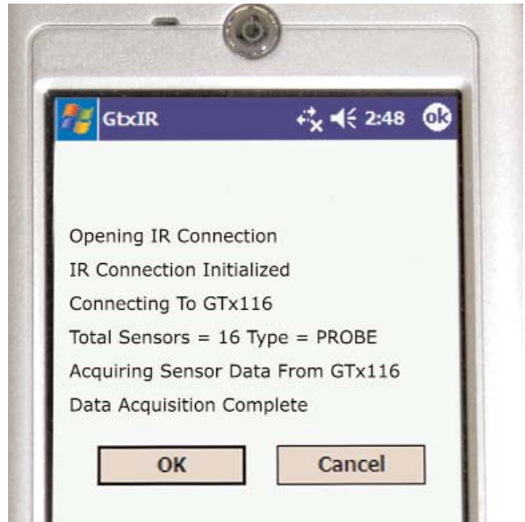
Figure 26. Typical PDA Display of EB-Link Initial Data Acquisition Screen
